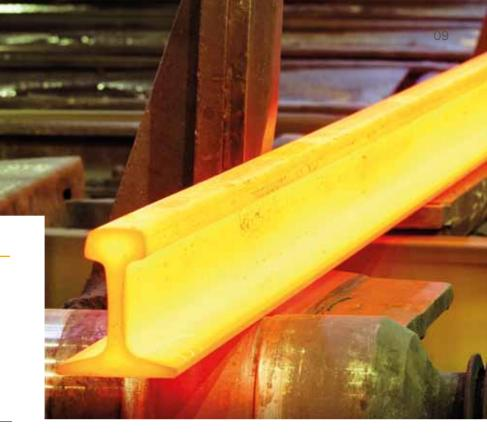
We supply a wide range of rails in sizes from 33 to 113 kilograms per metre (kg/m), and in a variety of steel grades. With some of the world's most advanced technology at our disposal, we can produce rails to all existing standards, including those with very strict dimensional tolerances and in lengths of up to 100 metres for high-speed tracks.
